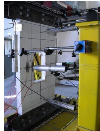
Fig. 6: Arrangement of LVDT
