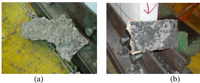
Fig. 16: Failure mode of the wall panels with openings strengthened with CFRP pattern 2 in (a) tension face and (b) compression face.
