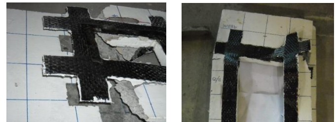
Fig. 14: Failure mode of wall panels with openings strengthened with CFRP pattern 1 in compression face.
